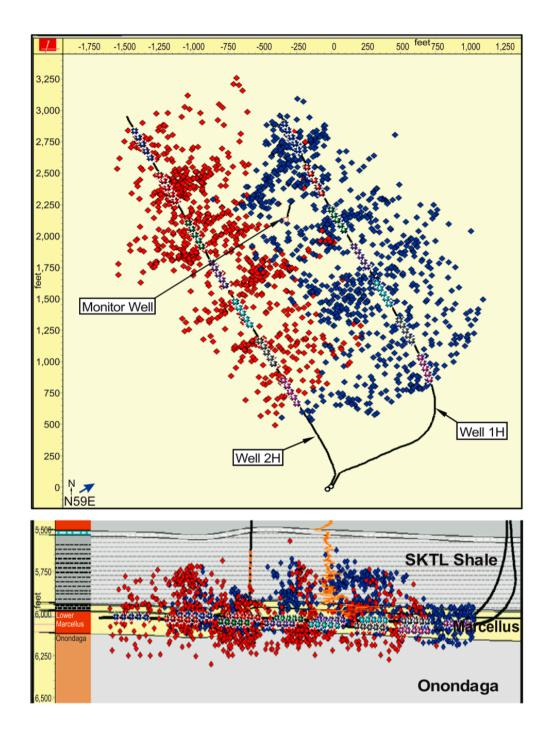
Figure 10Microseismicity associated with the fracture process from two<br/>adjacent horizontal wells (from Warpinski 2012)
