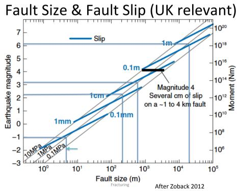
Figure 20 Fault dimensions for a variety of Earthquake magnitudes (after Zoback and Gorelick 2010)
