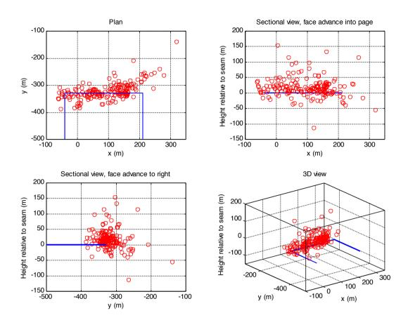
Figure 11b Microseismicity recorded using in-seam techniques from Coventry Colliery (Styles et al 1997)
