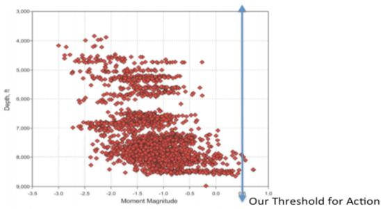
Figure 17 'Normal' microseismic activity from US fracking (after Warpinski et al 2011)
