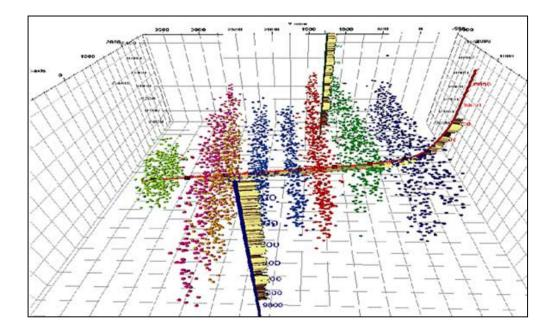
Figure 6 Microseismic clouds for a sequence of stimulations, which start at the furthest extent of the casing (left) and progressively work inwards. The horizontal and vertical extents of the fractures are clearly delineated by this micro seismicity. (Schlumberger 2007)
