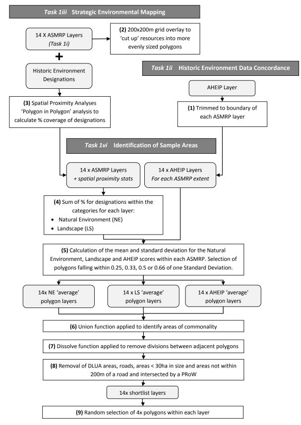
Figure 16 Flow diagram of methodology
