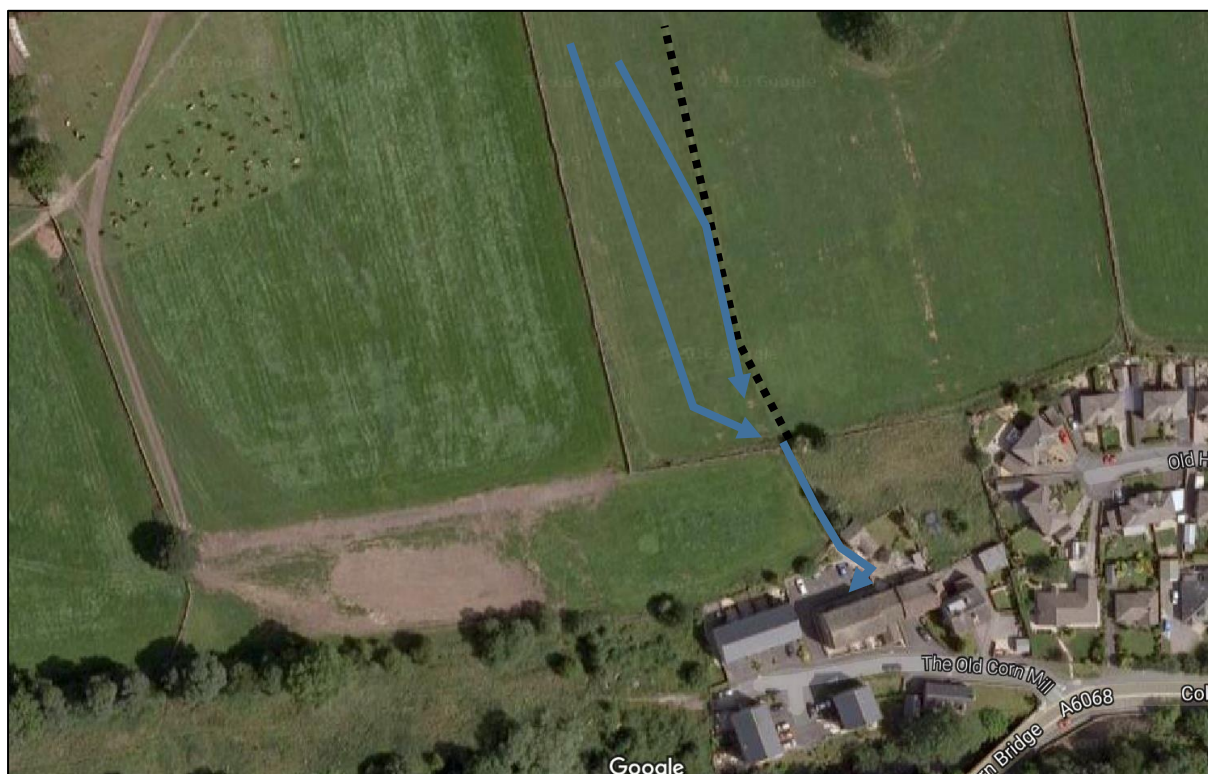
Figure 8.7 Mechanism of flooding at The Old Corn Mill
