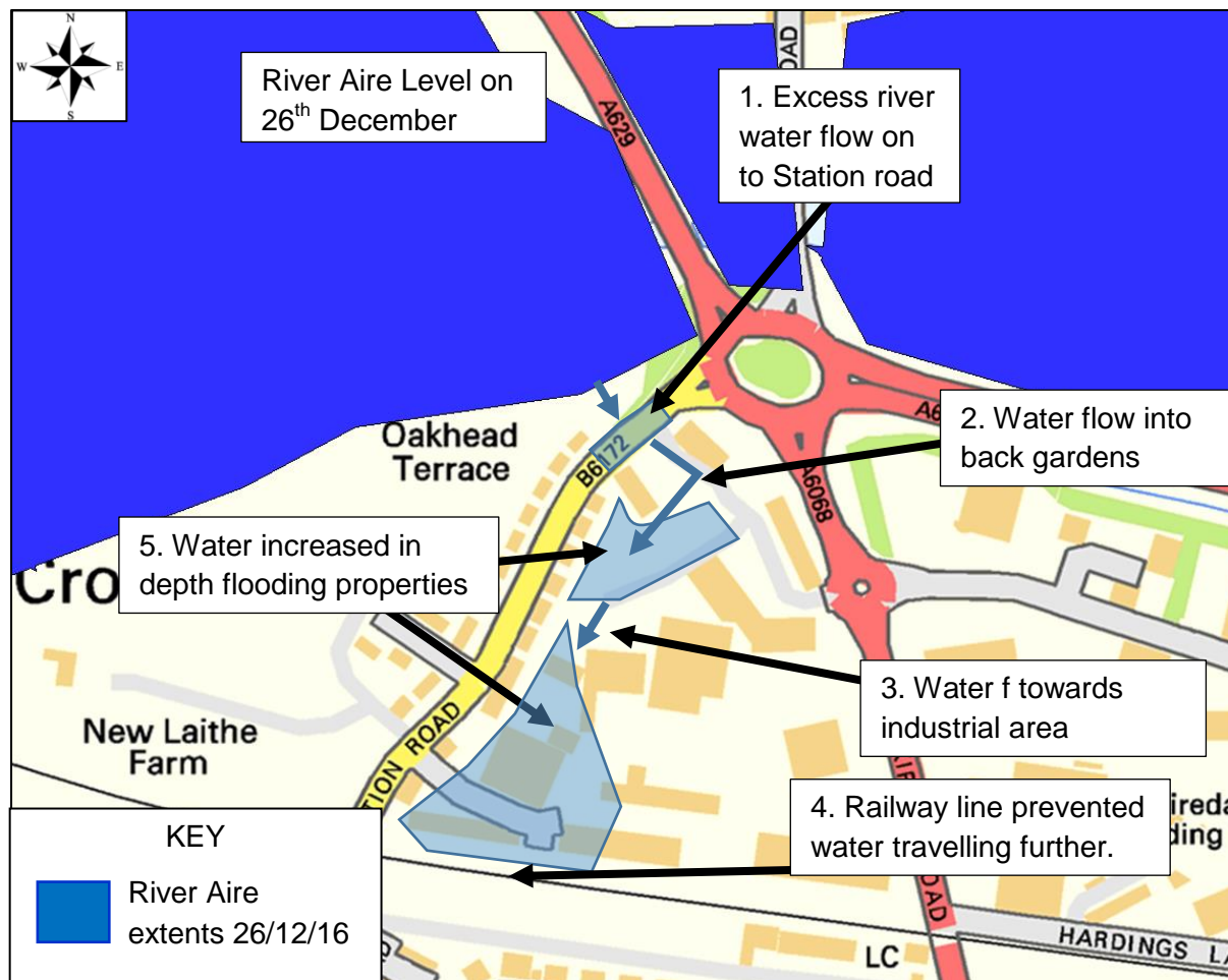
Figure 7.7 Mechanism of flooding on Station Road
