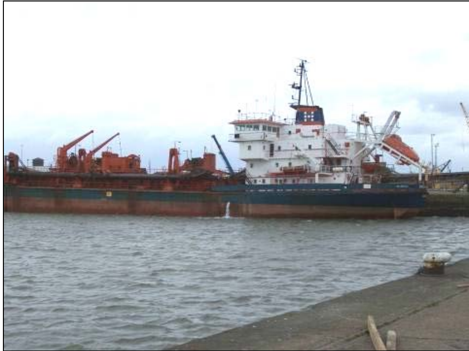
Photograph 1: Hanson dredger Arco Beck tied up at Alexandra Dock, Port of Hull. The ship has a reported load capacity of 4900 tonnes and draft of 6.51m (Courtesy of Humber Sand and Gravel Ltd.)
