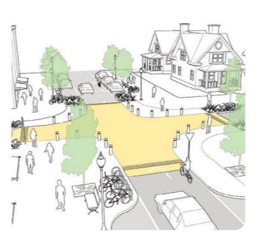
Raised table to reduce vehicle speed and improve users' experience.
