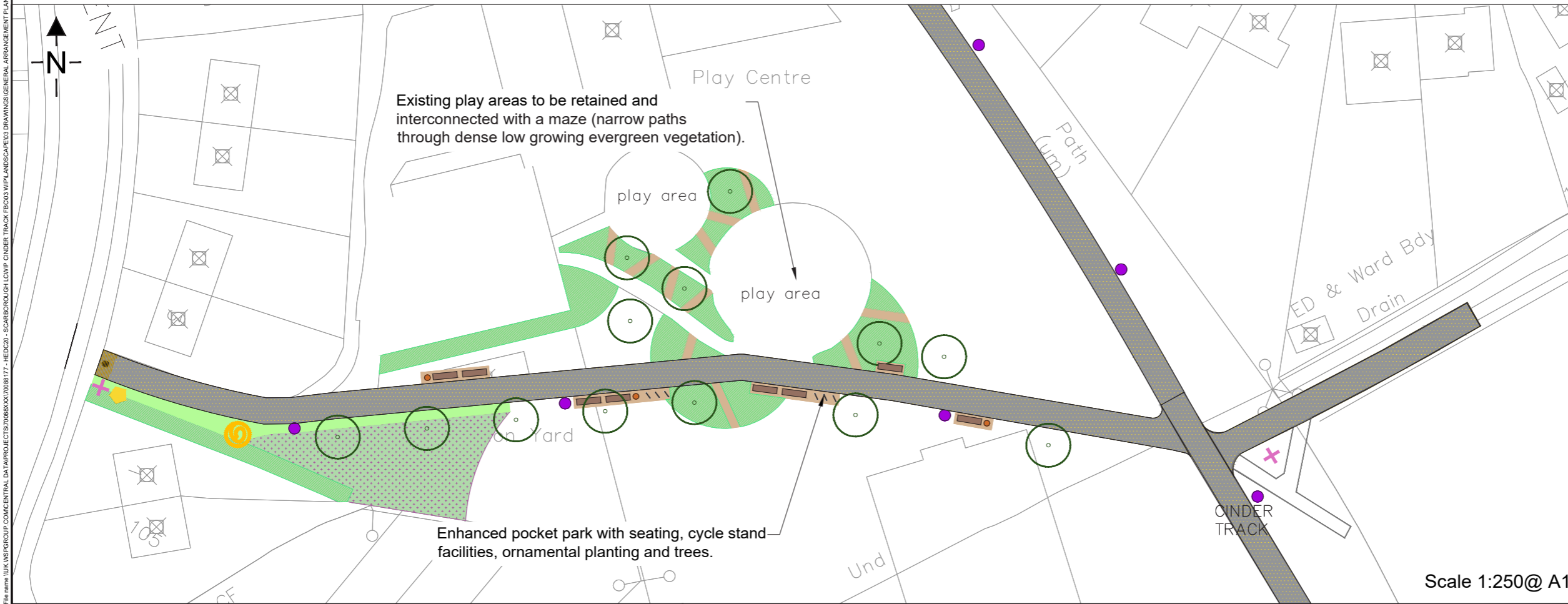
raised zebra crossing with consistent colour surface to promote branding of Cinder Track. Surface Colour red, orange or terracotta. Exact colour TBC at next stage
