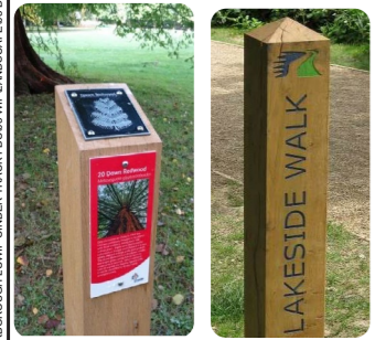
Wooden activity trail and wayfinding posts that act as bollards to restrain vehicular access, navigate and inform people at public realm
