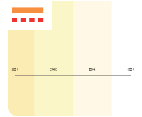
Bat friendly lighting Using warm light colours such as 2200K or 2700K that is considerate of the sensitive needs of nature and wildlife.
