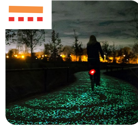
STARPATH technology to create wayfinding walkways - Spray on solution - Potential for use in combination with motion sensor street lighting along the corridor and links.
