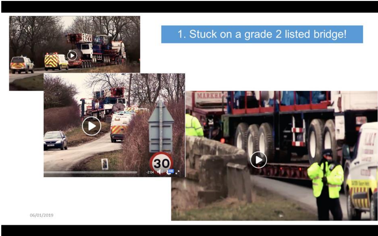
Figure 2 – Low loader grounded on top of Grade II Bridge
