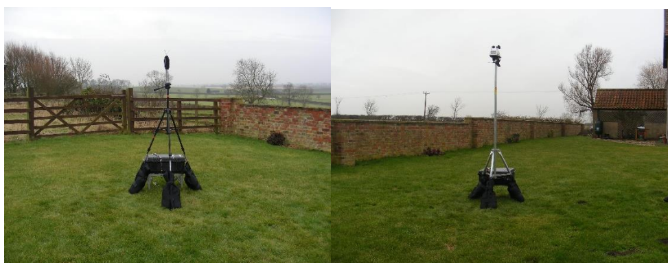
Figure 16.1. Baseline Noise and Weather Monitoring at Alma House
