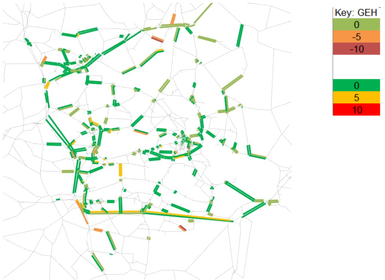
Figure 5-3 - GEH Statistic of Modelled Flow vs Observed Count by Direction - PM Peak
