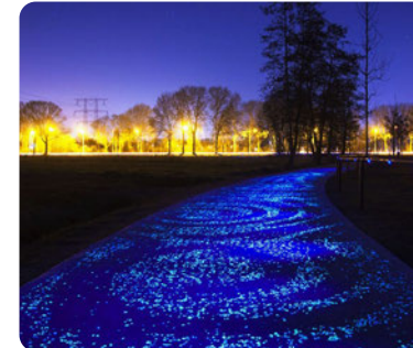
Star Path spray on solution on tarmac paths to aid wayfinding (pro-teqsurfacing.com)
