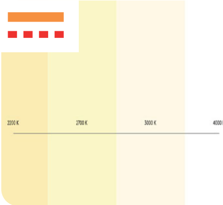
Bat friendly lighting Using warm light colours such as 2200K or 2700K that is considerate of the sensitive needs of nature and wildlife.
