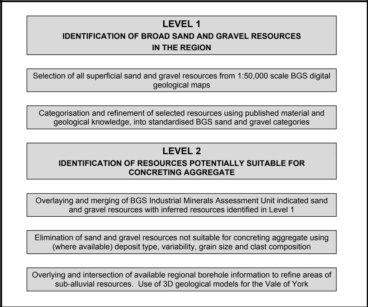
Figure 1. Key steps in sand and gravel resource selection and refinement
