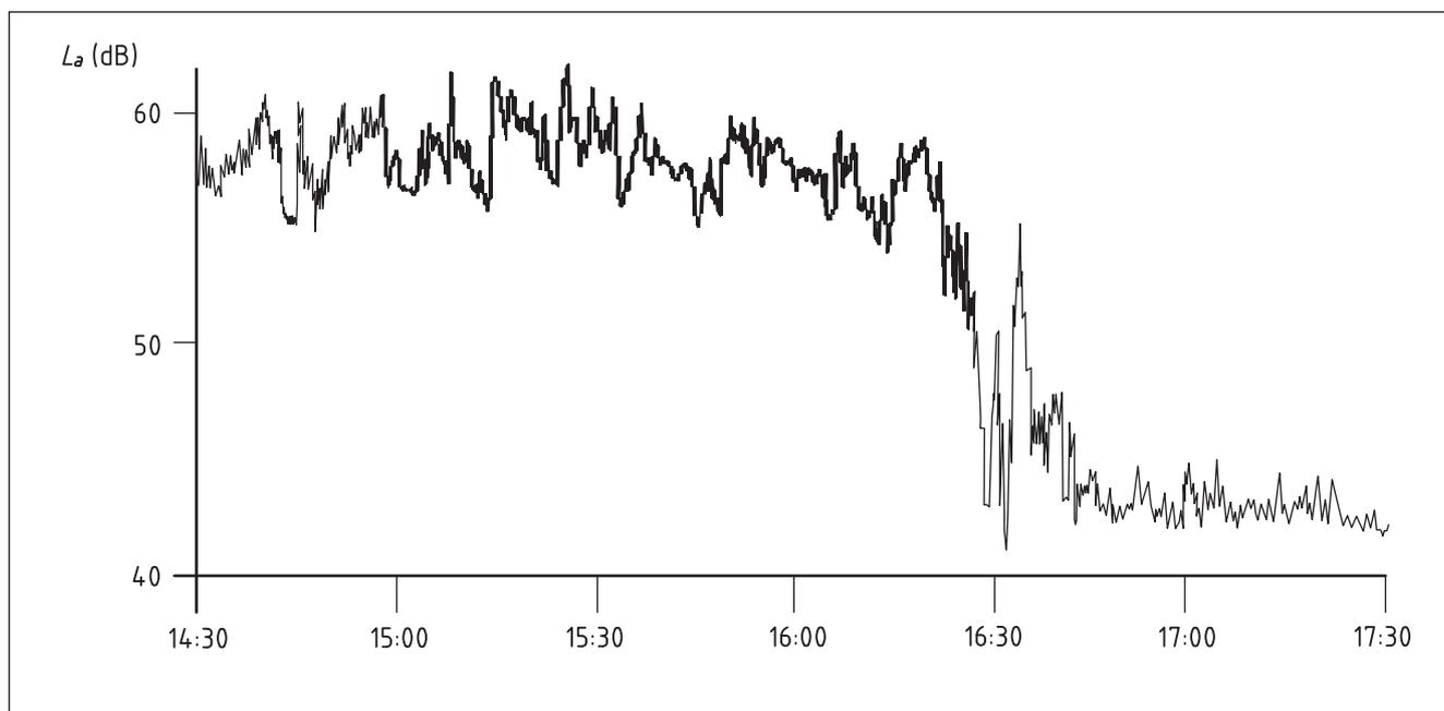
A subjective assessment of the impulsivity was considered inadequate to establish an appropriate rating penalty, so the reference method was used. The first half-hour period was assessed, which found regular impulses, the most prominent of which had a level change of 26.5 dB and an onset rate of 212 dB/s<sup>-1</sup>. This event had a calculated prominence  $P$  of 8.6, resulting in an adjustment  $K_1$  of 8.7 dB. This was rounded to a rating penalty of 9 dB.
