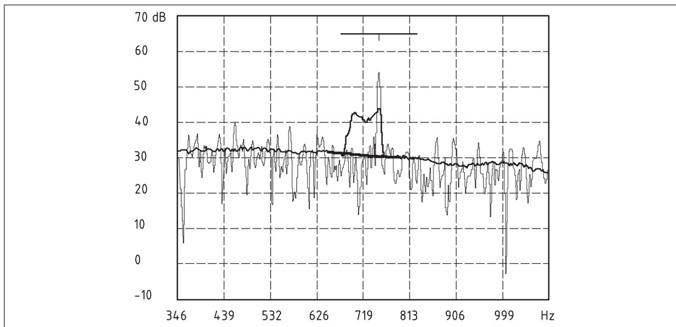
*NOTE* The graph shows both an averaged spectrum and an instantaneous spectrum. The tonal level may either be found by energy summation of the lines in the broad maximum in the averaged spectrum or by averaging the tone levels from a number of spectra measured with short averaging time, giving the same total averaging time.
