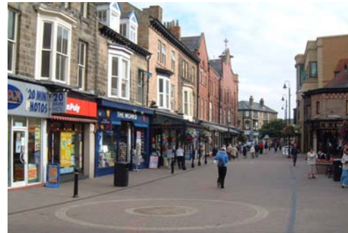
Oxford Street has a variety of roof types: eaves facing street; dormers; gables; parapet wall hiding roof; and hipped roofs.
