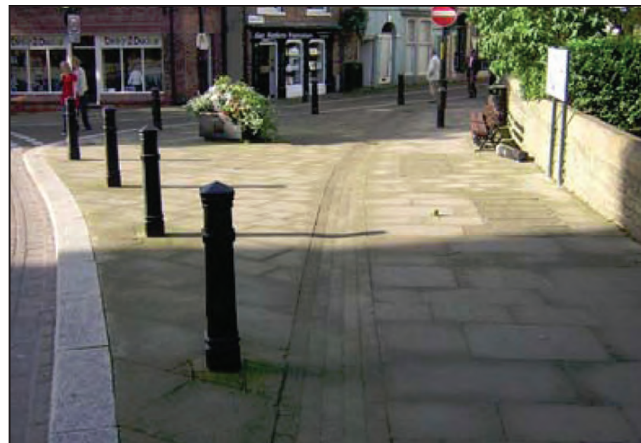
Figure 32: Bollards used to demarcate traffic from pedestrians without causing clutter in the streetscape.
