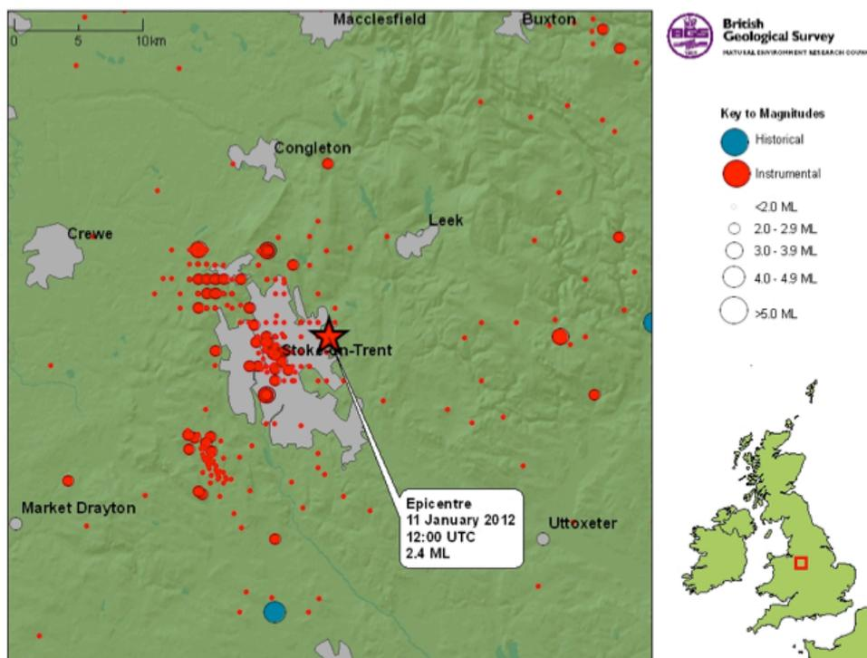
Figure 11a Seismicity recorded in the Potteries associated with coal mining including a magnitude 2.4 ML event (larger than the largest Blackpool Earthquake!)
