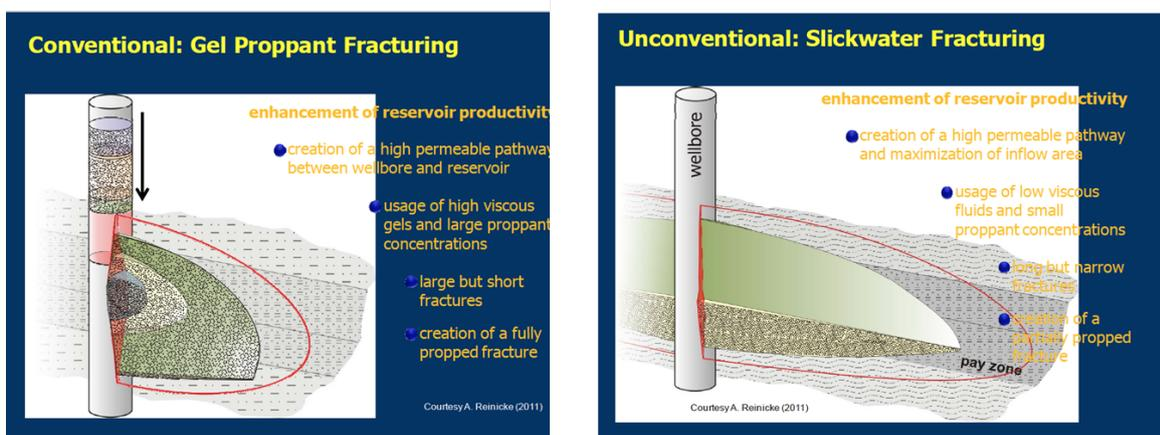
Figure 7 Gel and slickwater fracking
