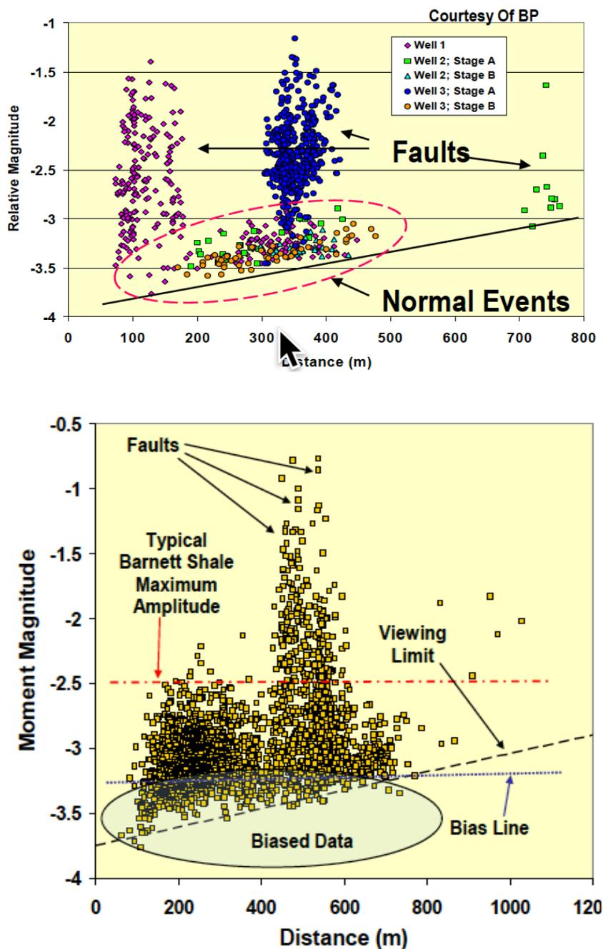
Figure 12 Microseismicity and its increase in magnitude as pre-existing faults are stimulated. Examples from the Barnett Shale.
