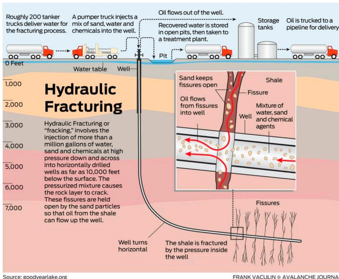
Figure 9 Schematic of the Hydraulic Stimulation (‘Fracking’) process
