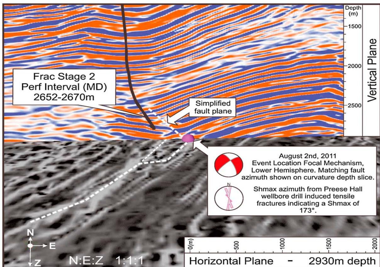
Figure 16. 3-D Seismic reflection data showing the relationship between the wellbore and the fault which was presumed to be the location of the induced seismicity. (Cuadrilla)
