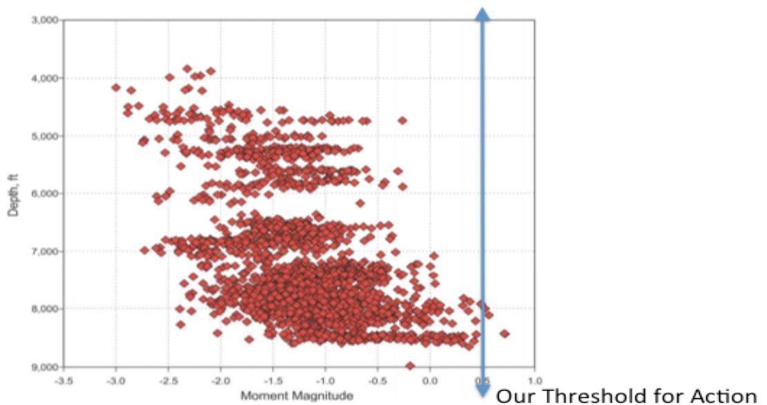
Figure 17 'Normal' microseismic activity from US fracking (after Warpinski et al 2011)
