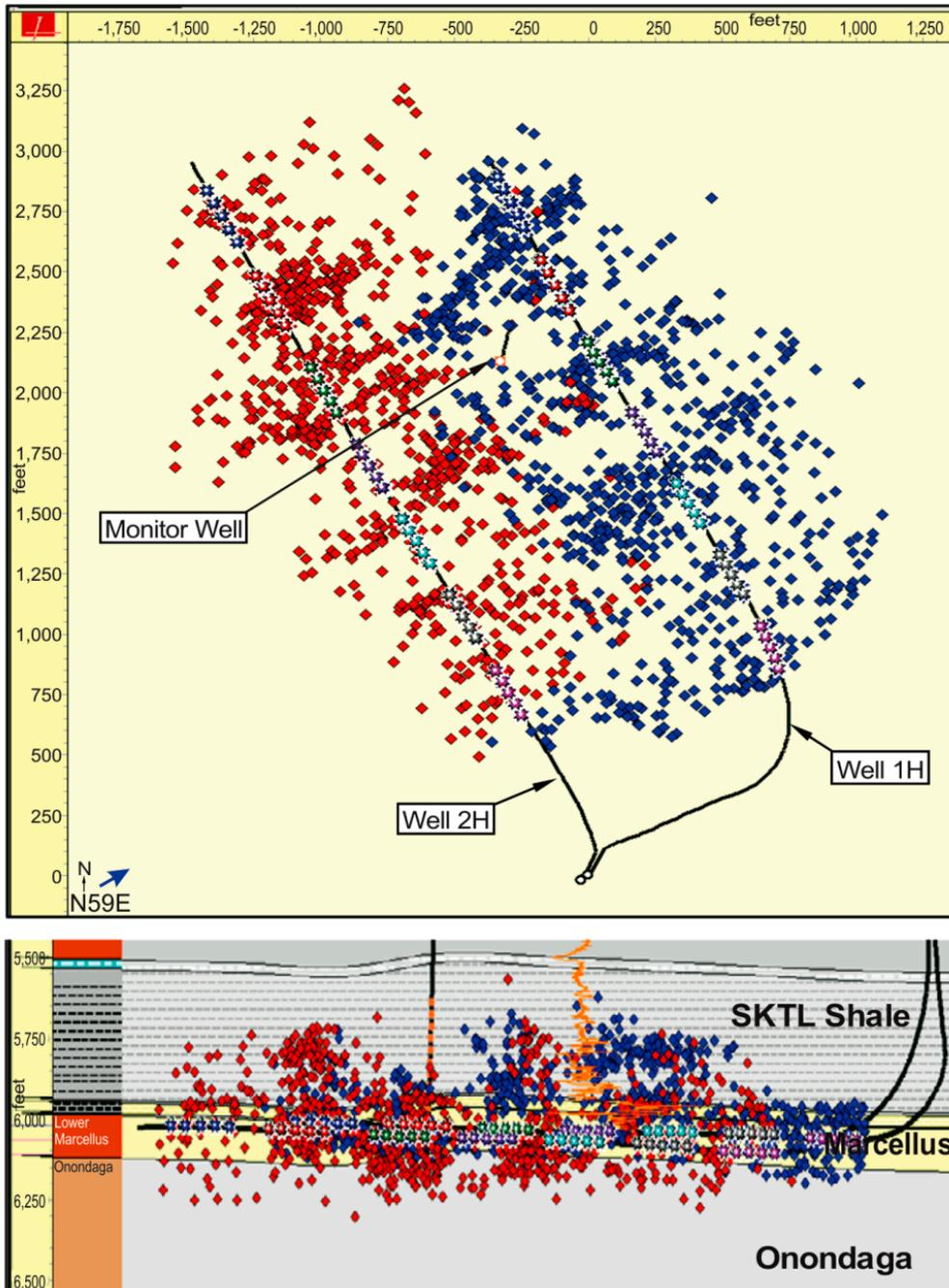
Figure 10 Microseismicity associated with the fracture process from two adjacent horizontal wells (from Warpinski 2012)
