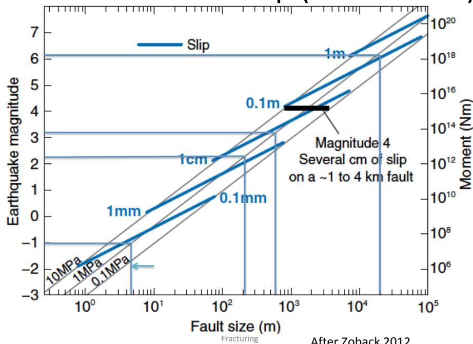
Figure 20 Fault dimensions for a variety of Earthquake magnitudes (after Zoback and Gorelick 2010)
