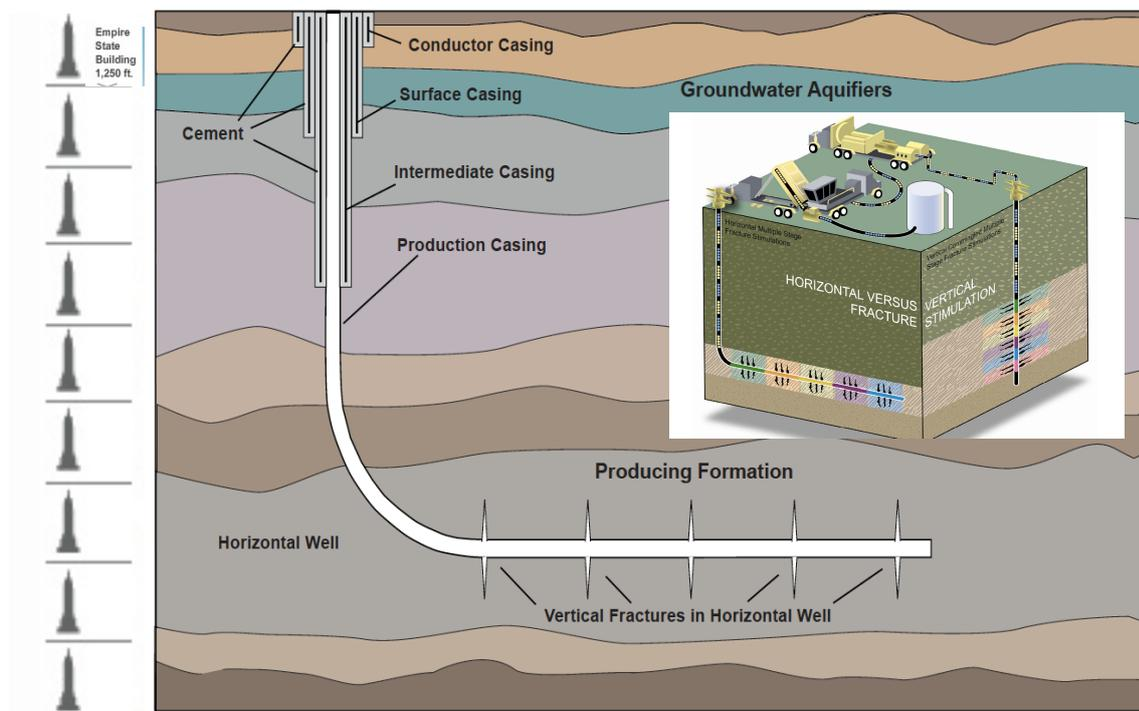
Figure 4 The Casing structure and the geometry of a hydraulic stimulation (fracking) process. Note that this is NOT to scale and that fracking typically occurs at c 3 km (10,000 feet) as shown by the multiple Empire State Buildings shown on the left. (Sundry sources)
