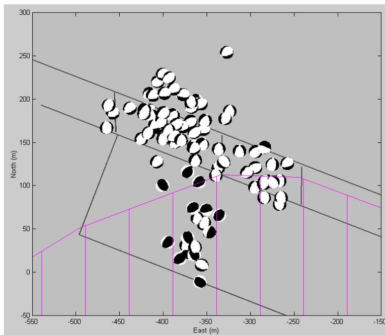
Figure 11 d Location of microseismic events and their source mechanisms during extraction at Asfordby Colliery, Note the normal faulting sources (white rugby balls), in the vicinity of the workings but thrust mechanisms (black rugby balls), lying above and south of the workings, considered to be associated with stimulation of activity on a pre-existing fault.
