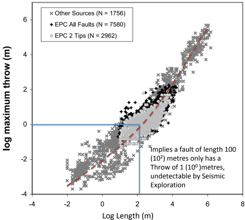
Figure 21. Relationship between Fault Length and Fault throw for faults measured underground in the East Pennine Coalfield (Bailey et al. 2002)
