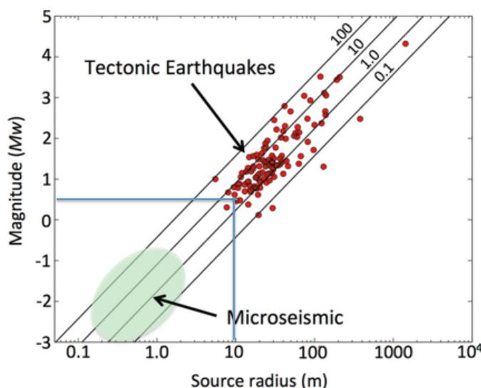
Figure 18 Discrimination between 'normal' microseismic events and induced (fault involved) seismic events and the 0.5ML threshold
