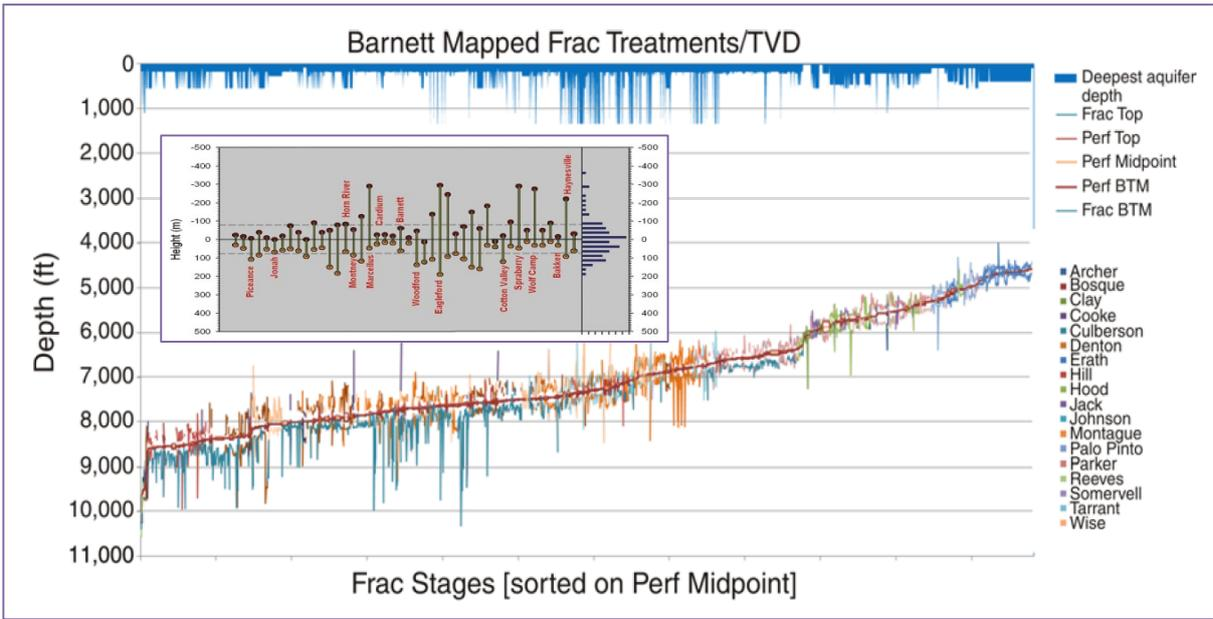
Figure 8. Vertical extent of hydraulically stimulated fractures with respect to aquifers and to the casing position (inset). After Warpinski et al (2012) and Maxwell (pers. comm).
